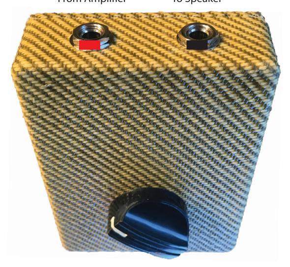
**IMPORTANT!** - Make sure your amplifier output is rated for the Impedance of the attenuator. If it is not, do not use. As this could cause damage to your amplifiers output transformer. You have been warned! I will not accept responsibly for improper use or hook up. Use with amplifiers rated over the wattage of the select attenuator is at your own risk!
