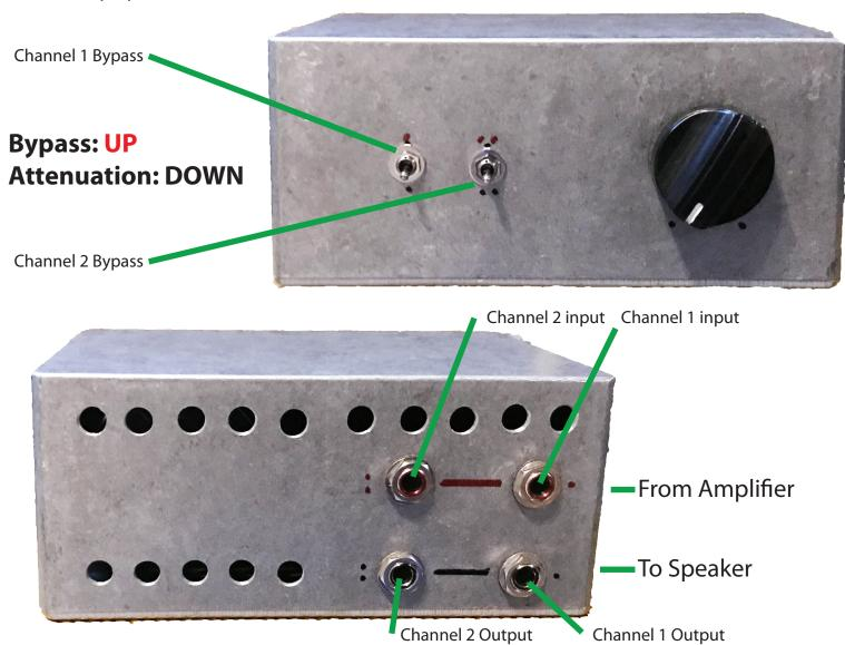
**IMPORTANT!** - Make sure your amplifier output is rated for the Impedance of the attenuator. If it is not, do not use. As this could cause damage to your amplifiers output transformer. You have been warned! I will not accept responsibly for improper use or hook up. Use with amplifiers rated over the wattage of the select attenuator is at your own risk!
